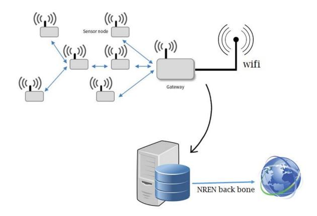
Figure 5: AWS network architecture
